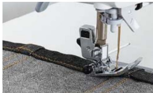
Thick denim folded into three layers for a flat fell seam Evenly sews thick fabrics effortlessly.
